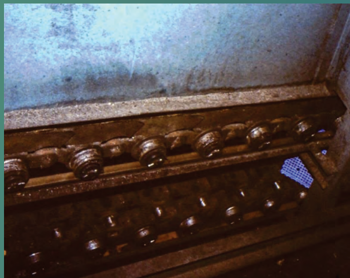
Any wear on the loaded side of the sleeve can be counteracted by turning the sleeve through 90° so as to present a new wear face.
